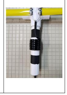
14. Attach the shorter 35-1/8" director element to the 3-way tee with a nylon wire tie on each side of the tee. Pull tight and cut flush.
